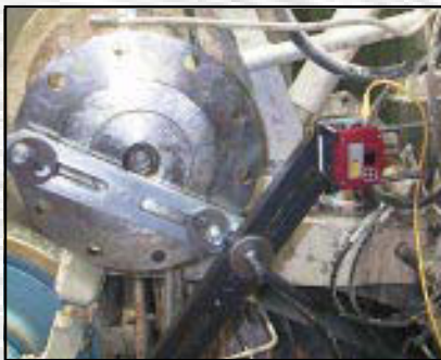
Alignment of offset mounted machines with Fixturlaser Shaft 200 and the cardan shaft fixture.
