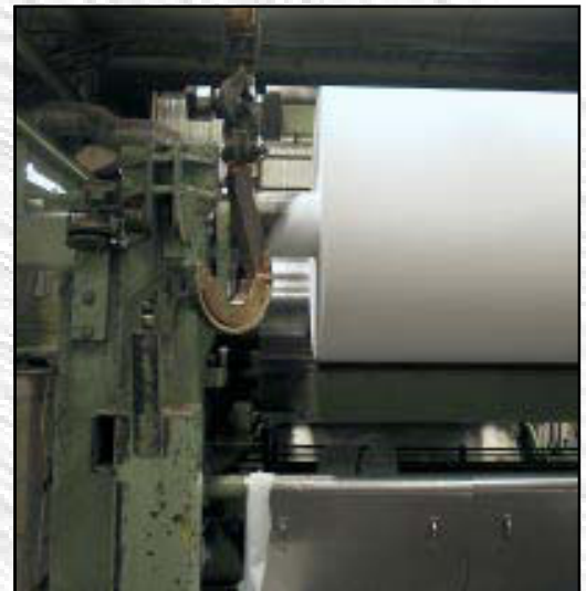
Roll parallelism in the winding section is crucial in order to control the quality of the finished roll and ultimately the sales result.
