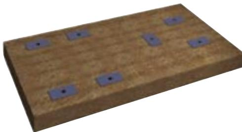
The flatness of a foundation is crucial for the machines. They will, otherwise, suffer from strains in their casing.
