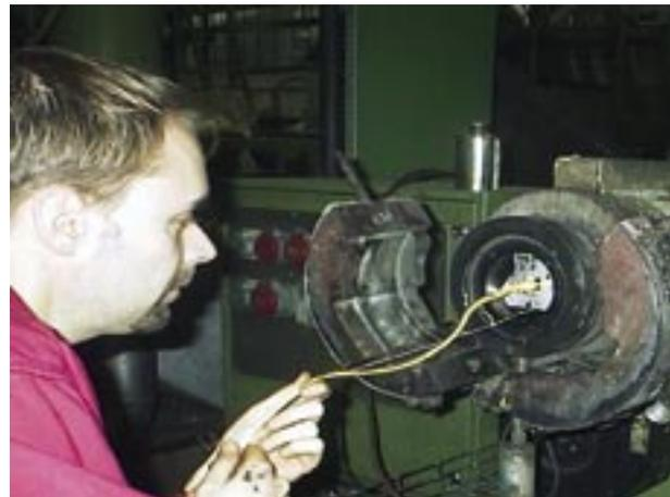
Registration of measurement values using the Fixtur Laser Extruder fixtures.
