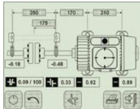
The measurement result is presented on the screen with all relevant information. Angular and offset errors, as well as the current foot positions of the movable machine are displayed. All values are continuously updated during adjustment, guiding the operator to a perfect alignment result.
