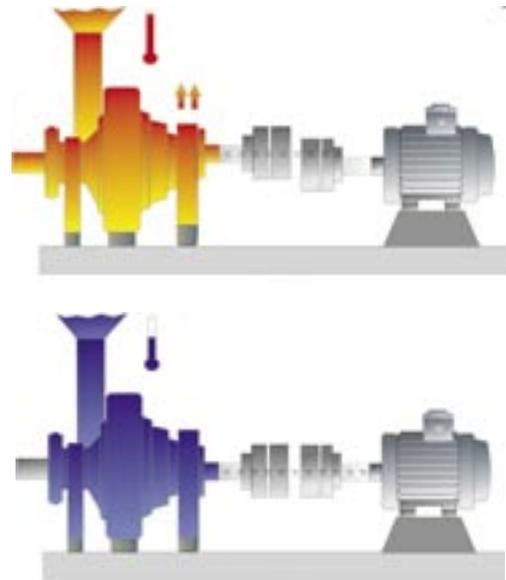
*Machines move and grow from offline to running conditions. The Fixturlaser Shaft series have the capability to measure and calculate with these specific deviation values.*
