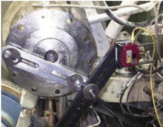
Alignment of offset mounted machines with Fixturlaser Shaft<sup>200</sup> and the cardan shaft fixture.
