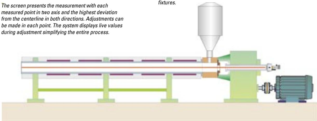
Extruder alignment system for precise measurement and alignment of the extruder barrel, according to the gear box's and the screw's axis of rotation.
