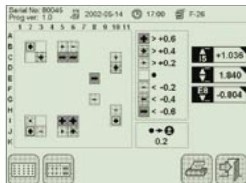
Above the documentation of how the flatness alignment process is displayed on the result screen and print out. As you can see, the distance between measurement points does not have to be equal, the choice is yours.
