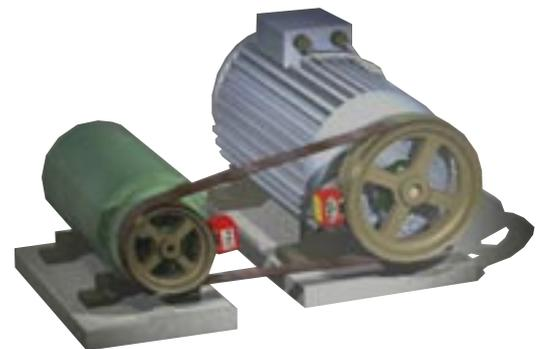
*The Fixturlaser PAT fixtures are used for aligning belt drives.*
