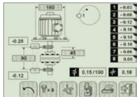
Vertical shaft alignment with Fixturlaser Shaft series. The result screen shows the current position of the motor and clearly advises necessary shimming.
