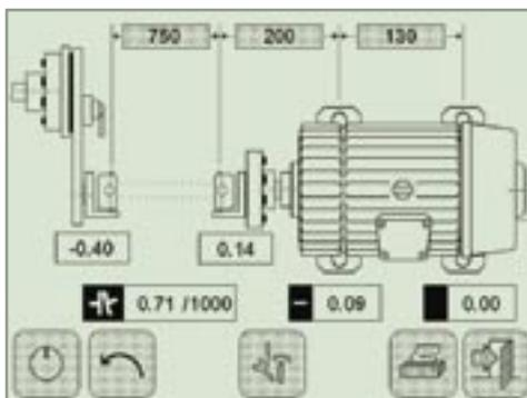
Alignment of offset mounted machines/cardan shafts follows the same procedure as for horizontal shaft alignment. The result screen tells us the position of the machine. The angular error of the coupling/cardan in this case is 0,71 mm/1000 mm.
