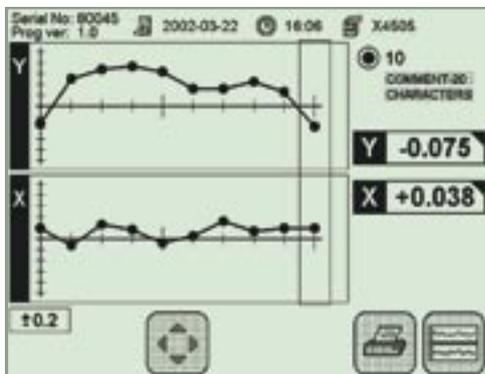
The screen presents the measurement with each measured point in two axis and the highest deviation from the centerline in both directions. Adjustments can be made in each point. The system displays live values during adjustment simplifying the entire process.
