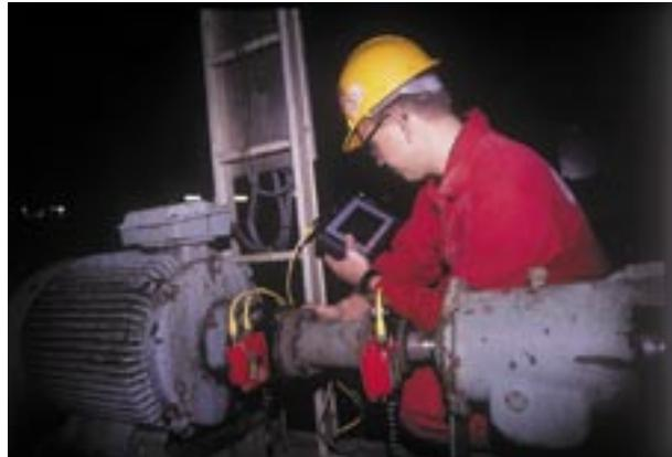
Misaligned machines contribute to huge costs in repair and production loss every year. By introducing preventive machine maintenance including regular alignment control, you minimize the number of unplanned stops due to machine breakdowns.
