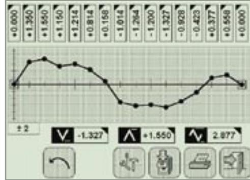
The screen displays a straightness measurement. The distances between the measurement points can be individual or equal. Each point can be named individually and commented for traceability purposes.
