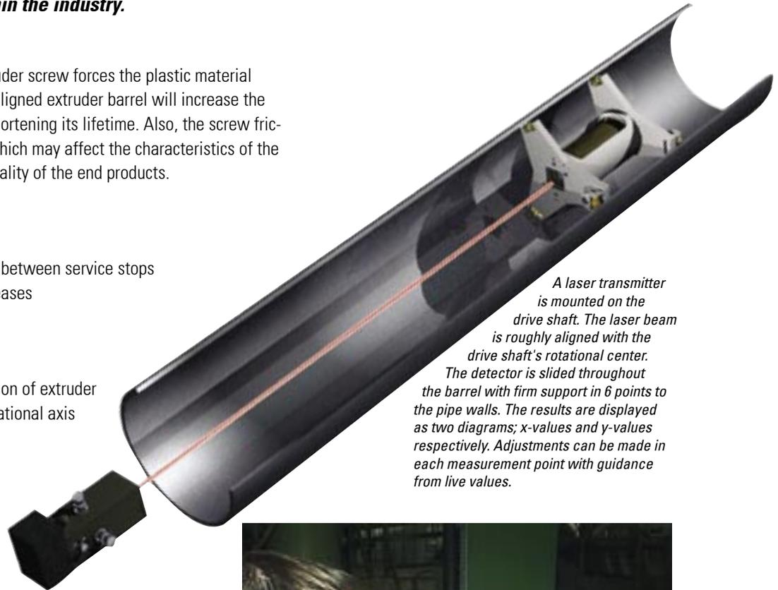
A laser transmitter is mounted on the drive shaft. The laser beam is roughly aligned with the drive shaft's rotational center. The detector is slid throughout the barrel with firm support in 6 points to the pipe walls. The results are displayed as two diagrams; x-values and y-values respectively. Adjustments can be made in each measurement point with guidance from live values.
