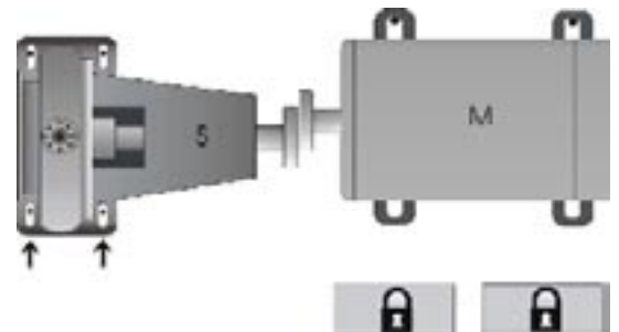
Restrictions in bolt holes.
