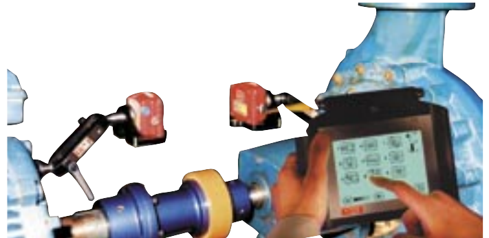
The Fixturlaser OL2R fixture mounted on motor and pump. Performing two measurements, one in offline mode and one in running mode, will give you the correction values for a precision alignment. The machine will be perfectly aligned considering all forces and movements from offline to running condition.
